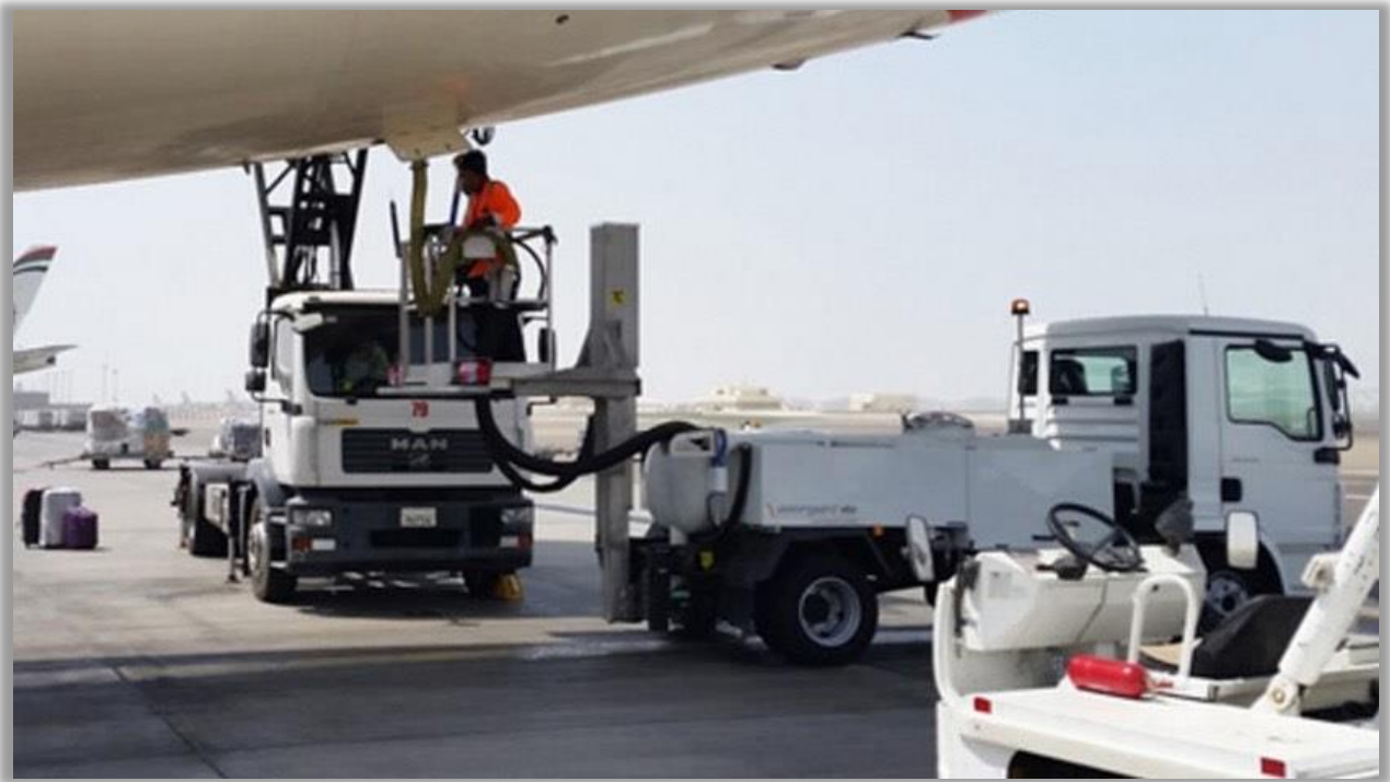
FLUSH: Airline lavatory service
